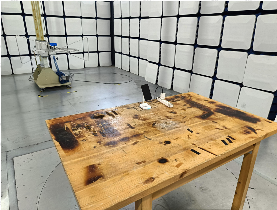
Photo of Radiation Emission Test
