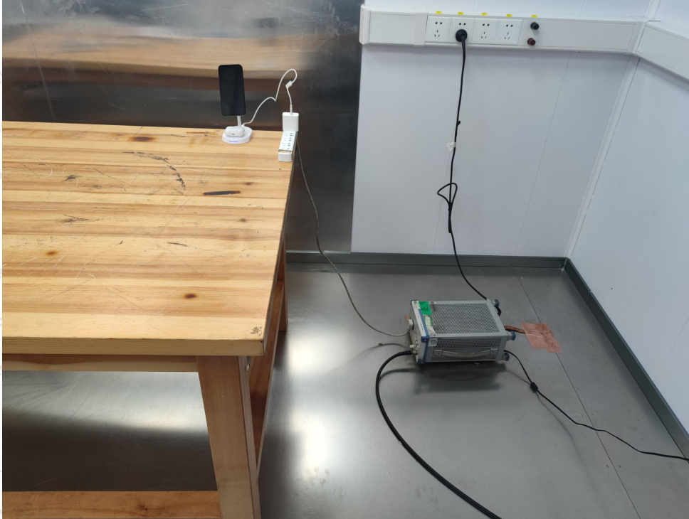
Photo of Conducted Emission Measurement
