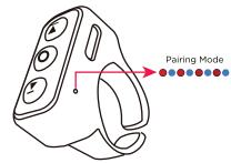
Go to the Bluetooth settings menu on your phone. Make sure the Bluetooth is turned on. Connect to the device listed as "WIRELESS PHONE CONTROLLER,"
