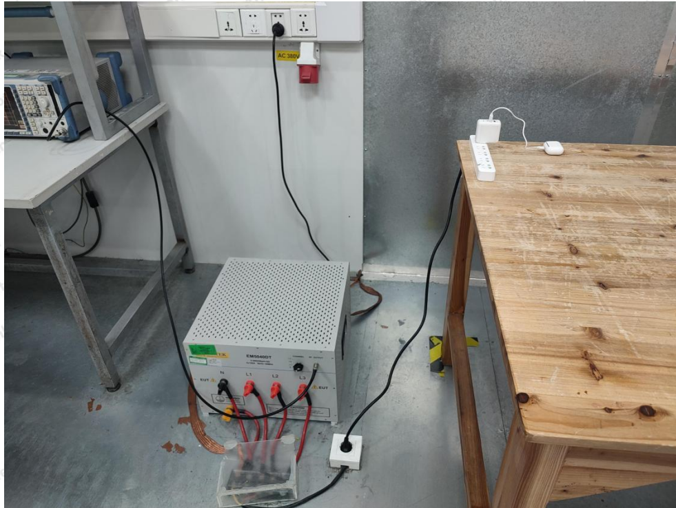
Photo of Conducted Emission Measurement
