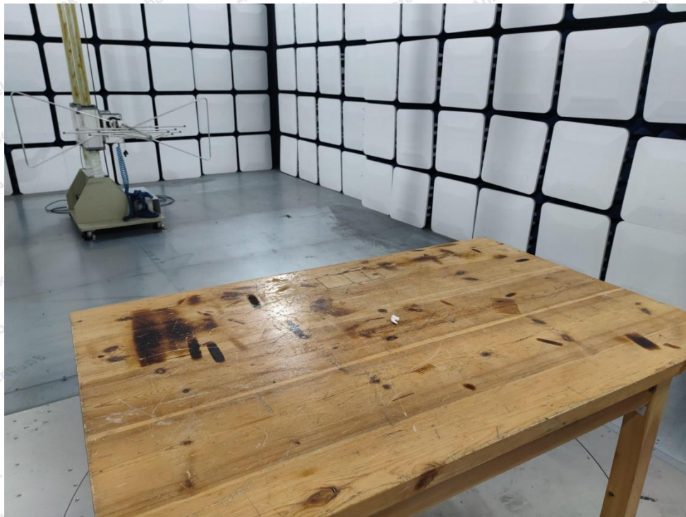
Photo of Radiation Emission Test
