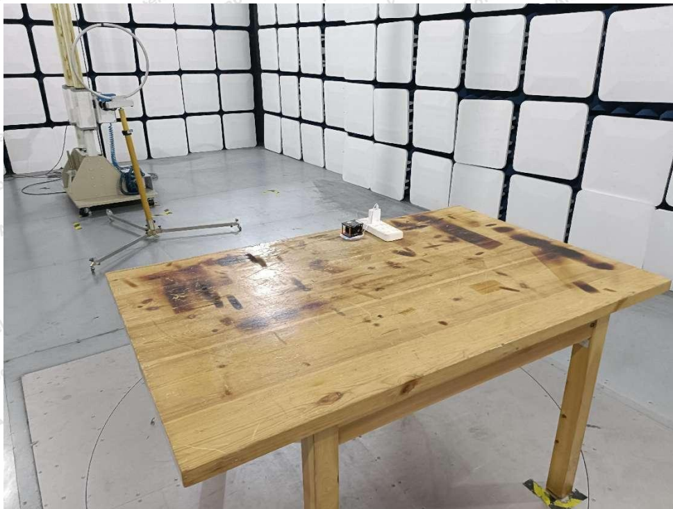
Photo of Radiation Emission Test
