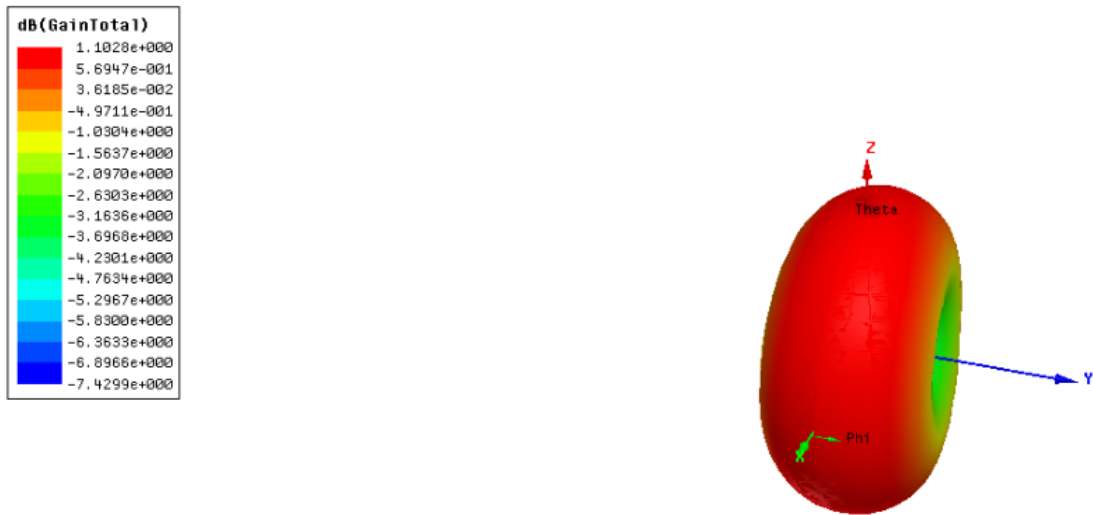
Figure 7. Antenna radiation pattern simulation
