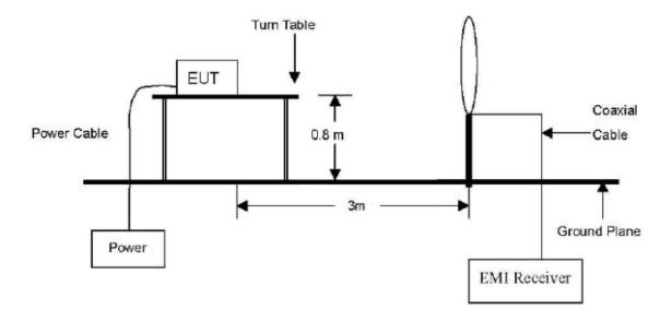
The diagram below shows the test setup that is utilized to make the measurements for emission from 30 Mb to 1 Gb emissions.
