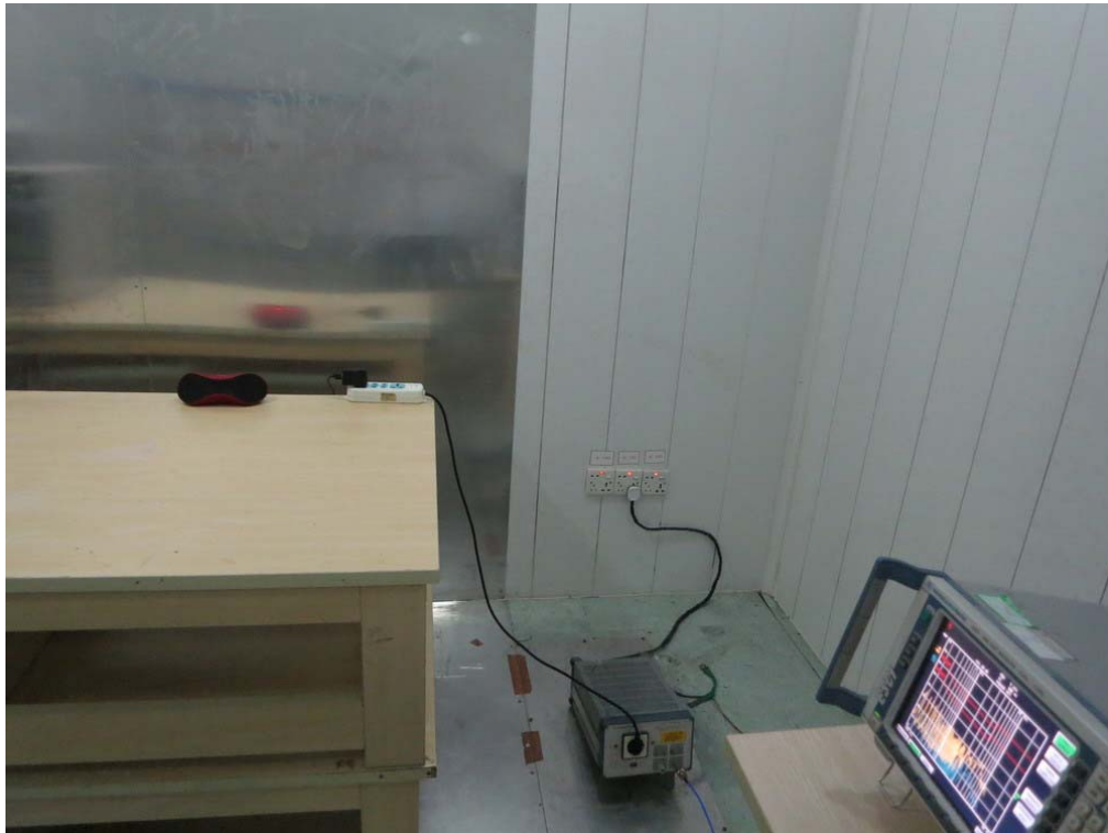
FCC RADIATED EMISSION TEST SETUP
