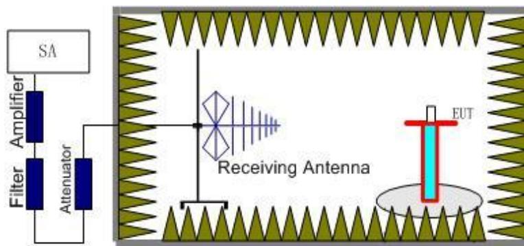
Radiated emissions measurements were made only at the upper, middle, and lower carrier frequencies of the PCS 1900 band (1850.2 MHz, 1880 MHz and 1909.8 MHz) ,GSM850 band (824.2MHz, 836.6MHz, 848.8MHz). It was decided that measurements at these three carrier frequencies would be
