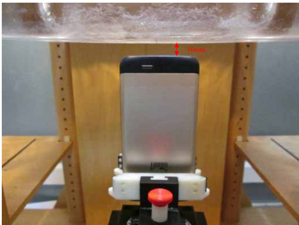
Body-worn Bottom Setup Photo (10mm)
