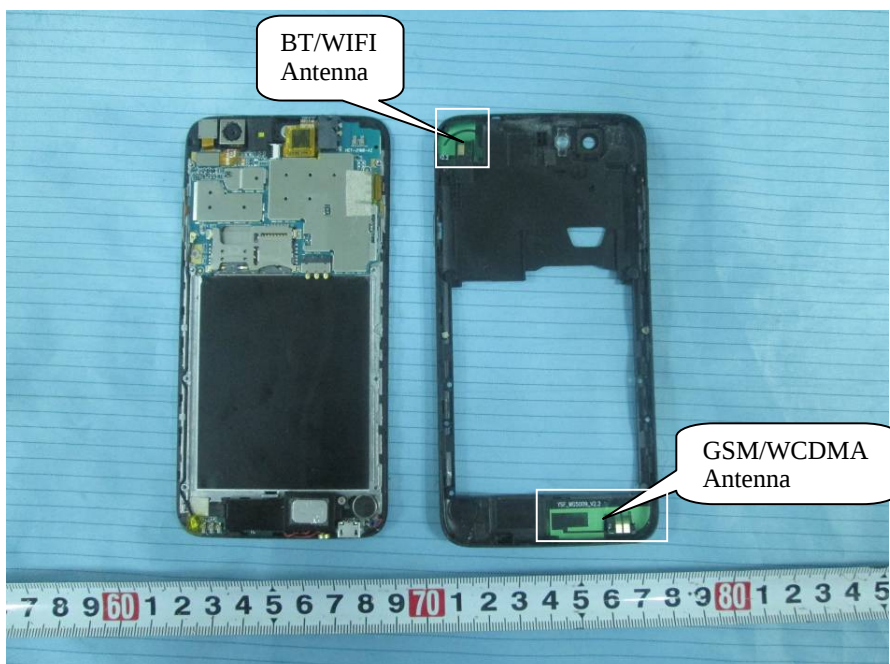
EUT – Bare Cover off View
