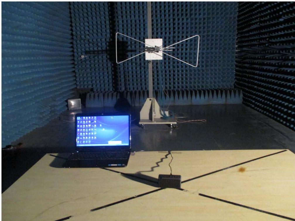
FCC RADIATED EMISSION TEST SETUP
