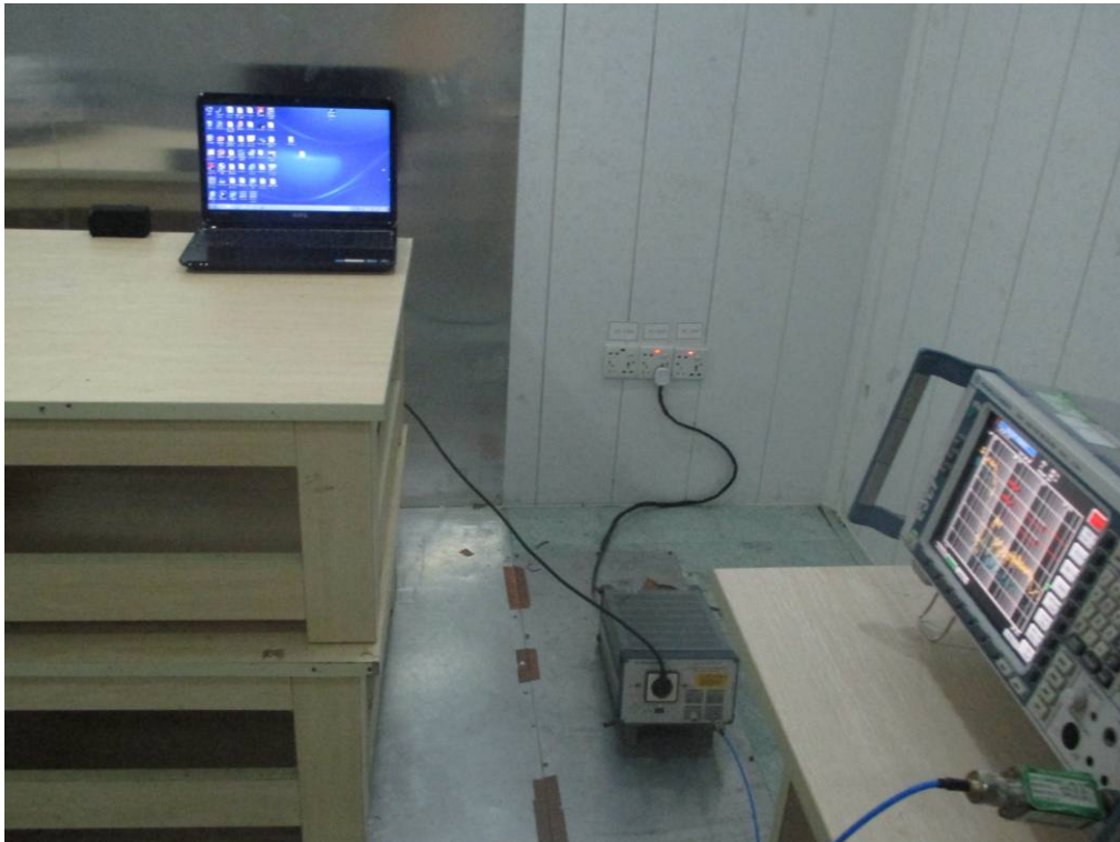
FCC RADIATED EMISSION TEST SETUP
