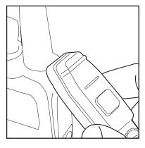
The LED indicator will light constant, when the LED flashes, its paired with your radio.
