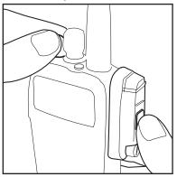
The LED on the FingerPTT is located on the inside.
