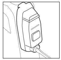
Take your Wireless FingerPTT and press and hold down both volume buttons for 5 seconds, until the LED flashes red 2 times.
