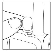
Push and hold the PTT button on the Gateway and then turn on your radio simutaneously.
