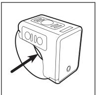
Take the Gateway and place the hook on the on top right side of the radio.
