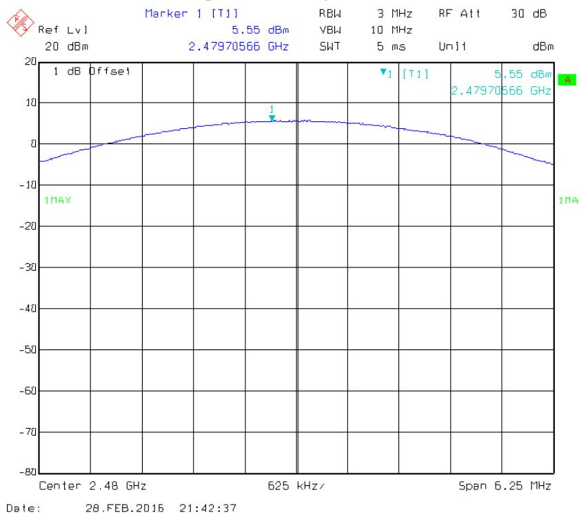
*EDR Mode (8-DPSK):***Output Power, Low Channel**
