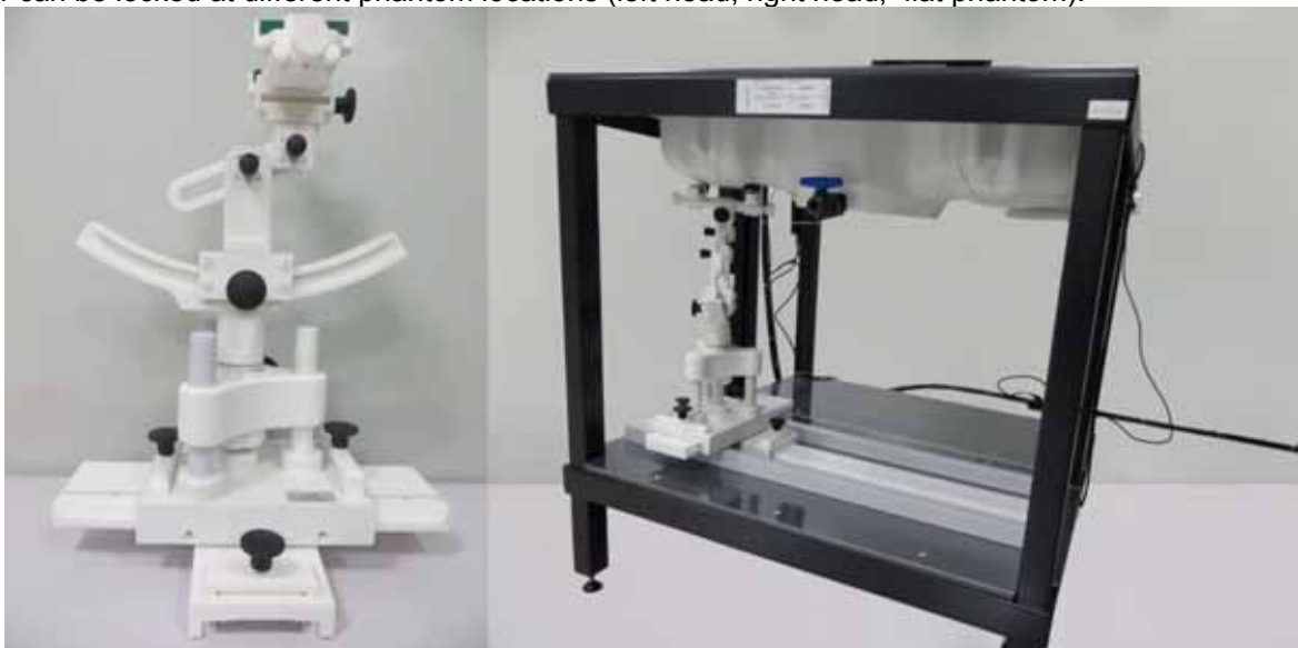
Device holder supplied by SATIMO
