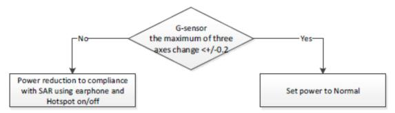
When the maximum of three axes change <+/-0.2, the user case MUST be mobile phone stay away from the body, but if it is>+/-0.2, it MAY be on the person's body, power reduction is on.
