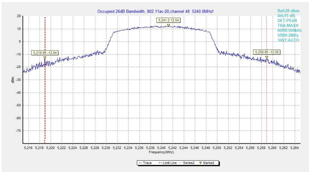
Fig.13 Occupied 26dB Bandwidth (802.11ac-HT20, 5240MHz)
