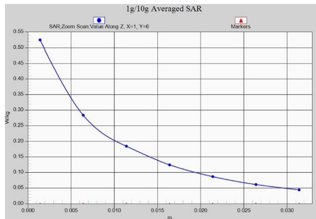
Z-Scan at power reference point (LTEB71)
