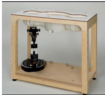
Picture C.10: SAM Twin Phantom
