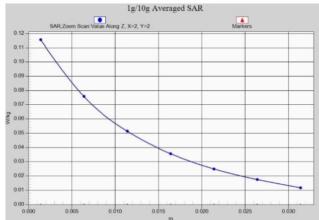
Fig. 1-3 Z-Scan at power reference point (1900 MHz)
