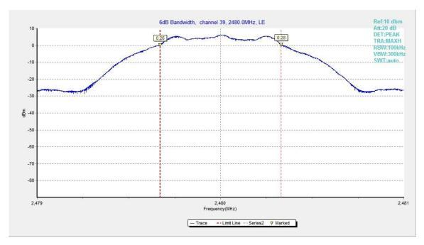
Fig.22. 6dB Bandwidth: GFSK, 2480 MHz
