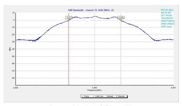
Fig.21. 6dB Bandwidth: GFSK, 2440 MHz
