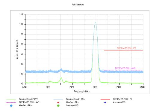
Fig.4. Frequency Band Edges: GFSK, 2480 MHz, Hopping Off, 2.45 GHz - 2.50GHz
