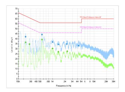
Fig.B.9.2 **AC Powerline Conducted Emission-Idle**
