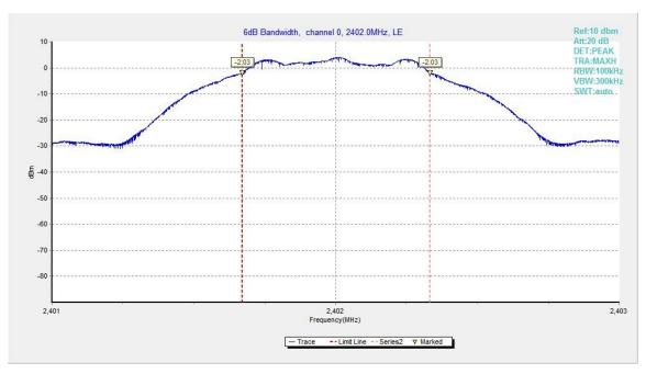
Fig.20. 6dB Bandwidth: GFSK, 2402 MHz
