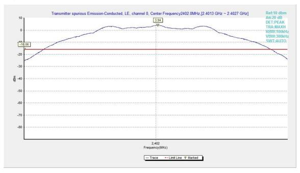
Fig.5. Transmitter Spurious Emission - Conducted: GFSK,2402MHz
