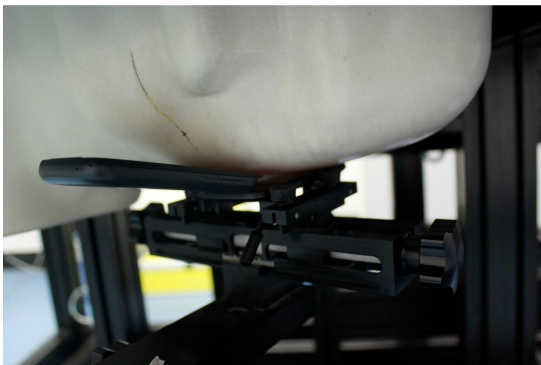
Picture 2: Left Hand Touch Cheek Position
