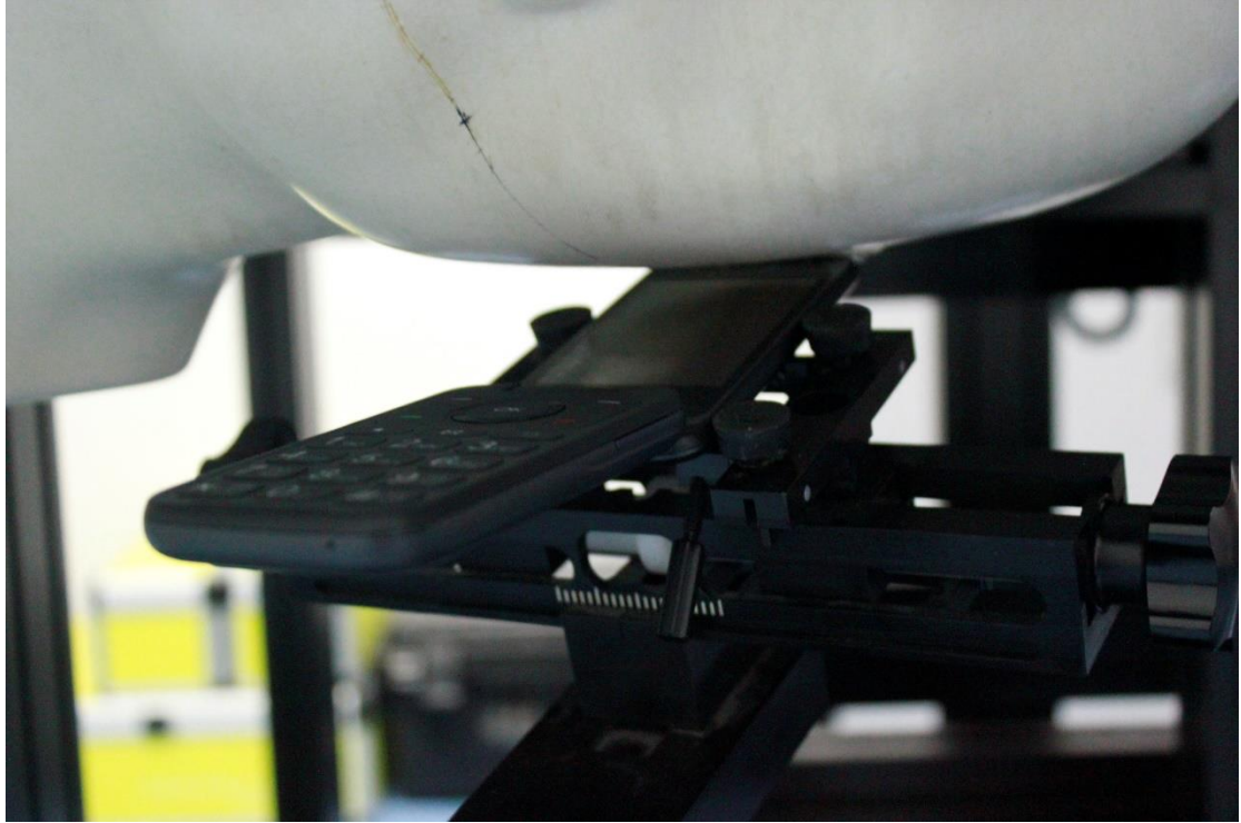
Picture 3: Left Hand Tilt 15° Position
