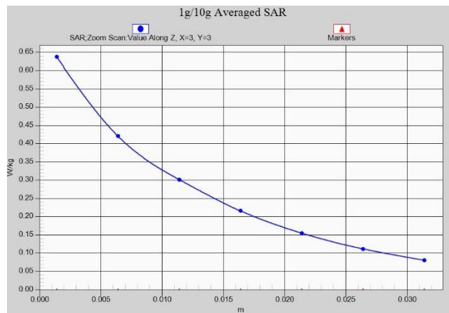
Fig. 1-19 Z-Scan at power reference point (LTE Band26)
