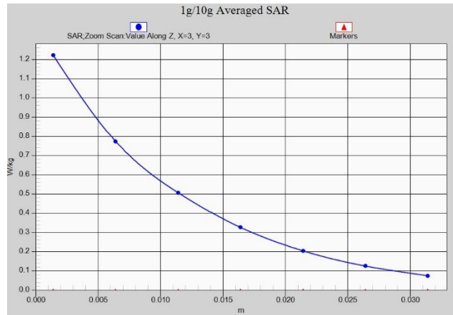
Fig. 1-16 Z-Scan at power reference point (LTE Band25)
