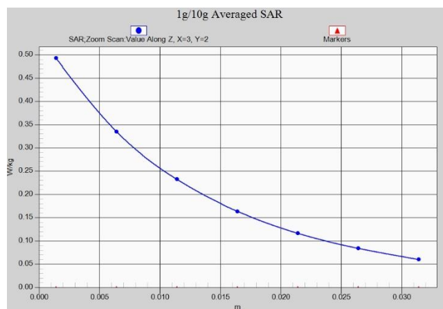
Fig. 1-8 Z-Scan at power reference point (WCDMA1700)
