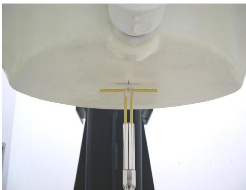
Picture 8.2 Photo of Dipole Setup
