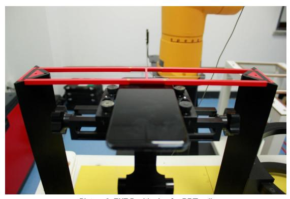
Picture 2: EUT Positioning for RF/T-coil
