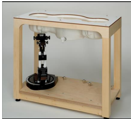
Picture C.10: SAM Twin Phantom
