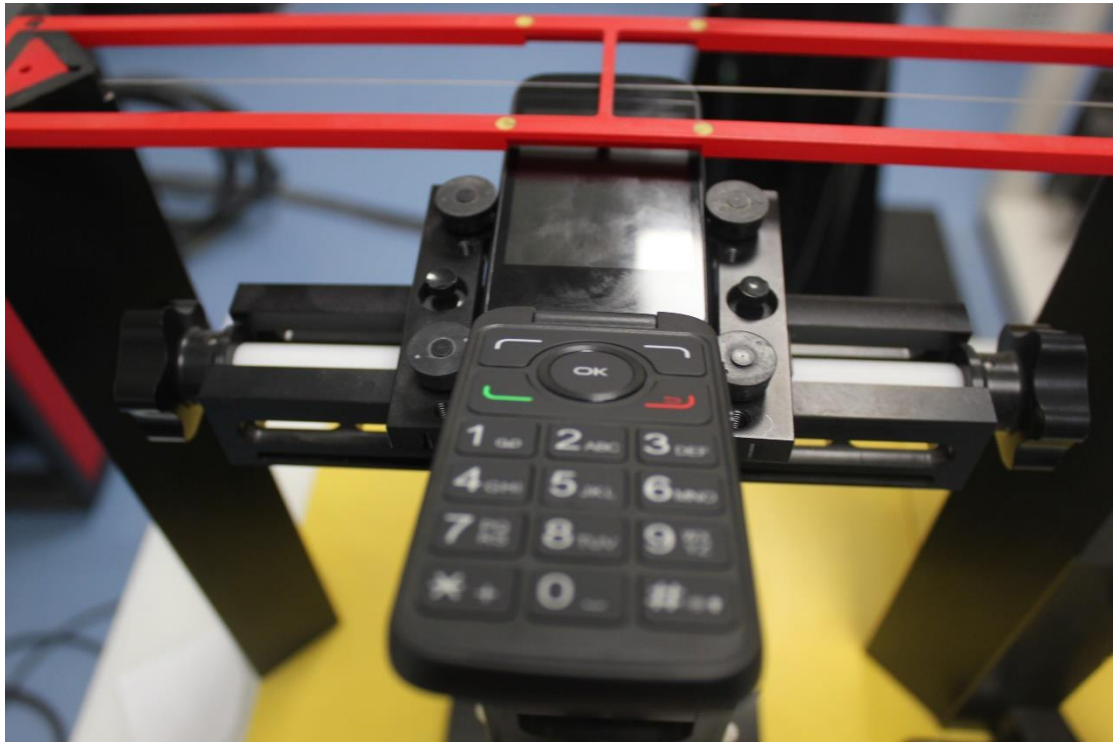
Picture 2: EUT Positioning for RF/T-coil
