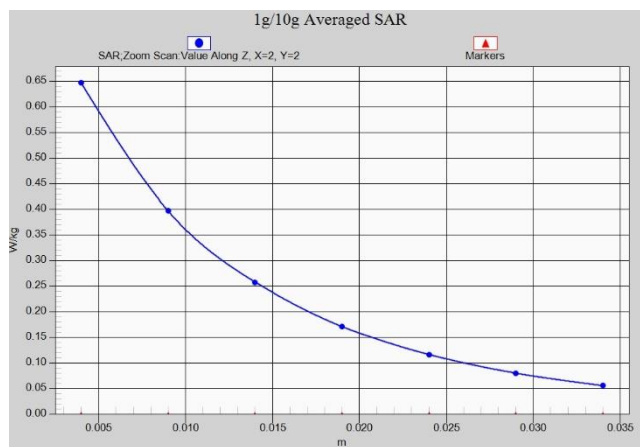
Fig. 1-14 Z-Scan at power reference point (CDMA BC0)
