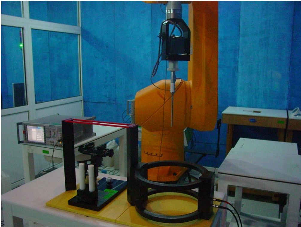
Picture A1: HAC T-Coil System Layout
