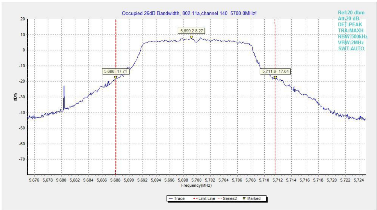
Fig.9 Occupied 26dB Bandwidth (802.11a, 5700MHz)
