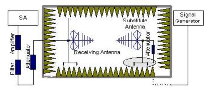
In the chamber, a substitution antenna for the frequency band of interest is placed at the reference point of the chamber. An RF Signal source for the frequency band of interest is connected to the substitution antenna with a cable that has been constructed to not interfere with the radiation pattern of the antenna. A power ( $P_{Mea}$ ) is applied to the input of the substitution antenna and adjust the level of the signal generator output until the value of the
