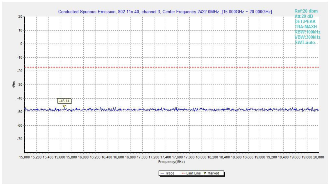
Fig.A.6.1.79 Transmitter Spurious Emission - Conducted (802.11n-HT40, Ch3, 15 GHz-20 GHz)
