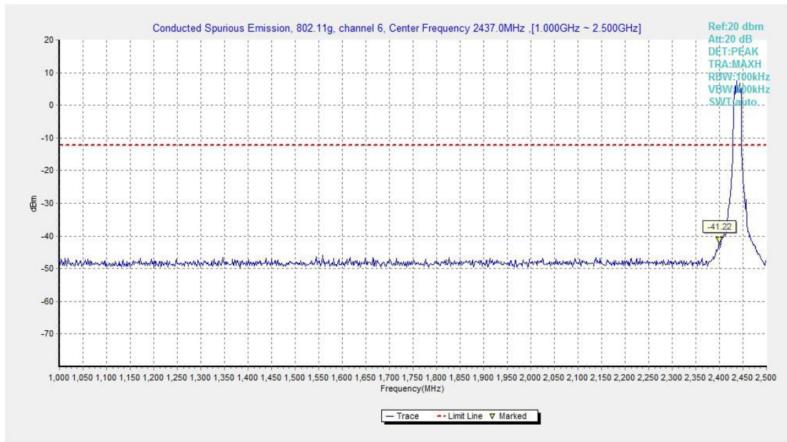
Fig.A.6.1.35 Transmitter Spurious Emission - Conducted (802.11g, Ch6, 1 GHz-2.5 GHz)
