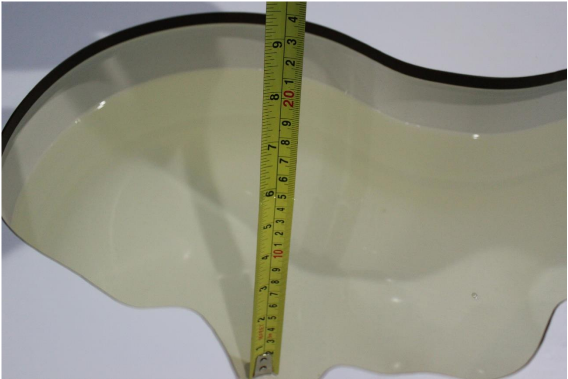
Picture 7-5 Liquid depth in the Head Phantom (5GHz)
