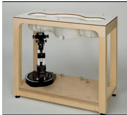
Picture C.10: SAM Twin Phantom
