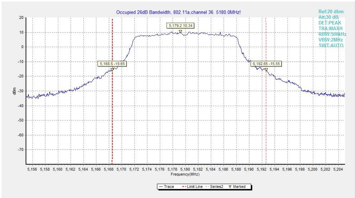
Fig.1 Occupied 26dB Bandwidth (802.11a, 5180MHz)
