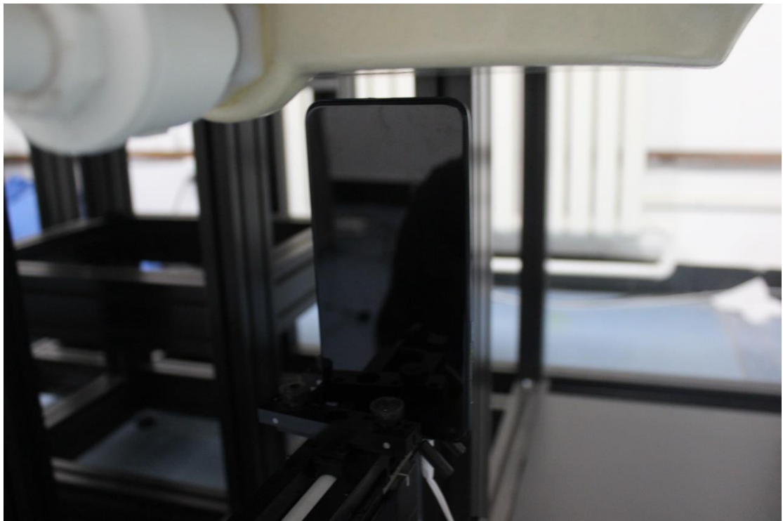
Picture 14: Bottom Headset 10mm
