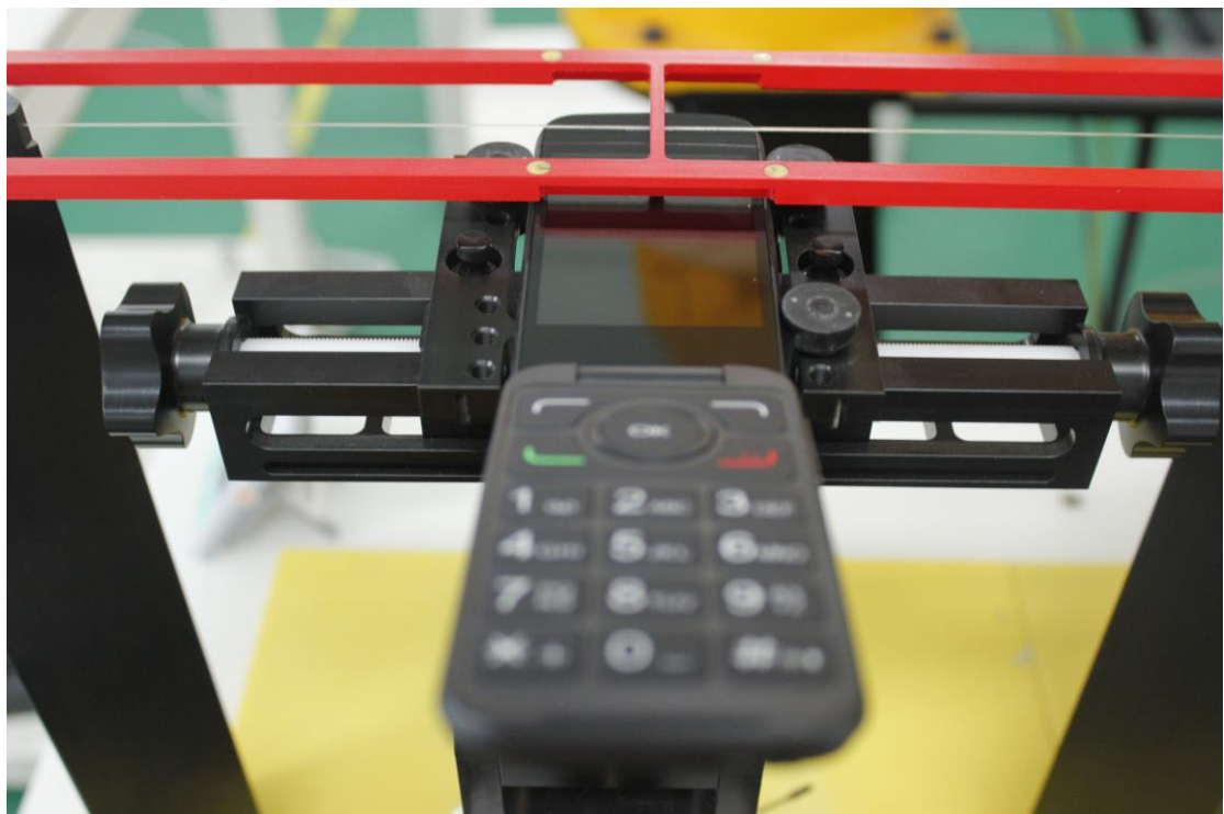
Picture 2: EUT Positioning for RF/T-coil
