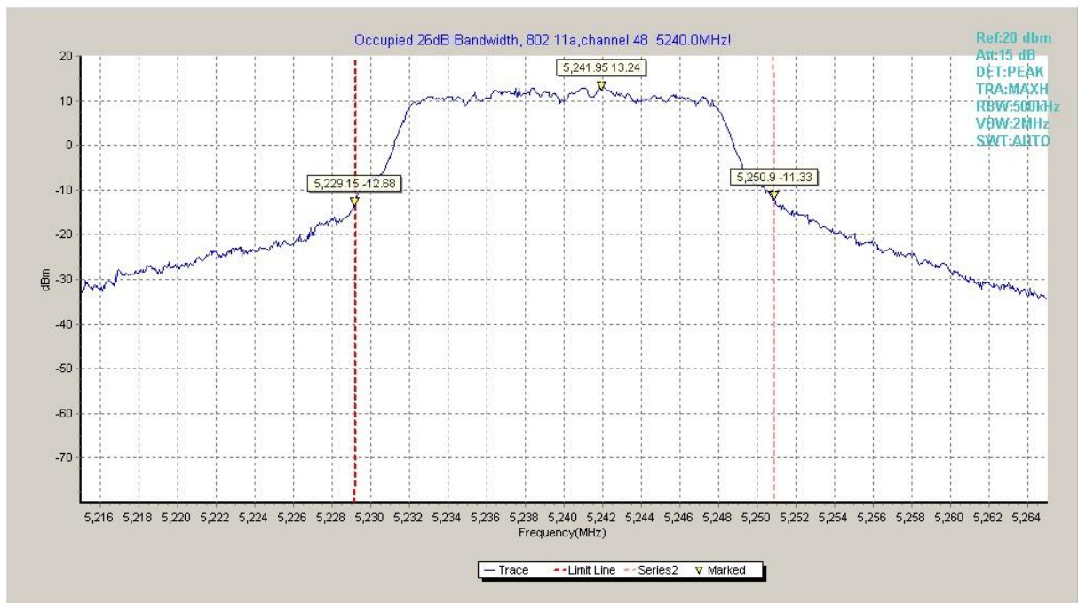
Fig.3 Occupied 26dB Bandwidth (802.11a, 5240MHz)
