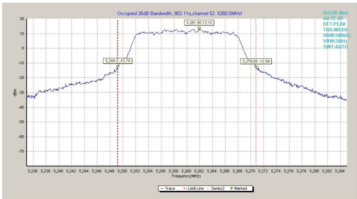
Fig.3 Occupied 26dB Bandwidth (802.11a, 5240MHz)
