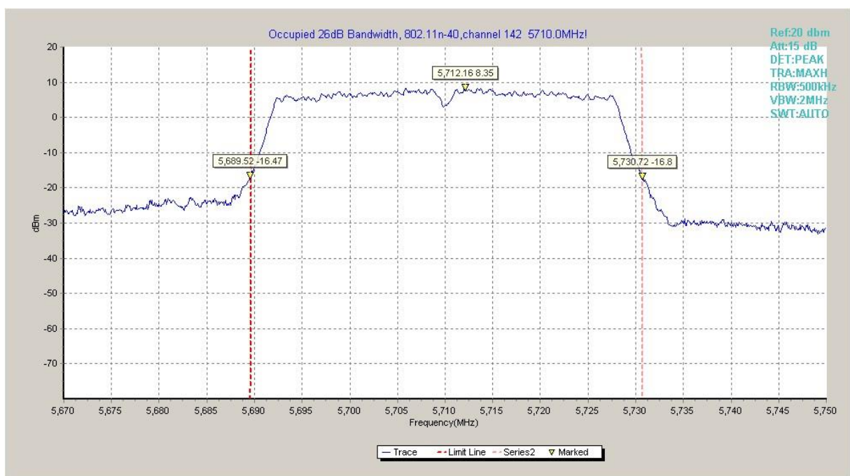
Fig.37 Occupied 26dB Bandwidth (802. 11n-HT40, 5670MHz)
