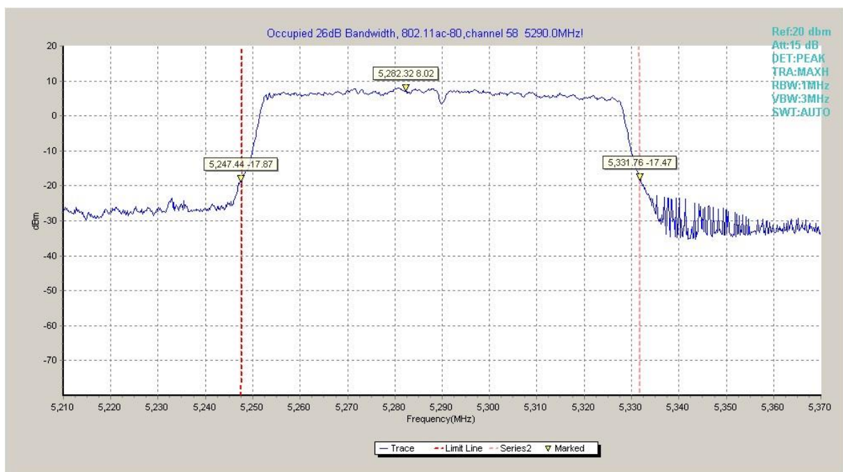
Fig.48 Occupied 26dB Bandwidth (802. 11ac-HT80, 5290MHz)
