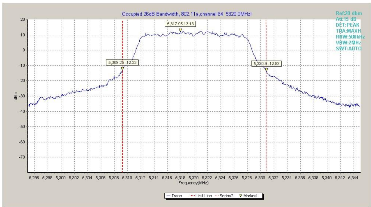
Fig.6 Occupied 26dB Bandwidth (802.11a, 5320MHz)
