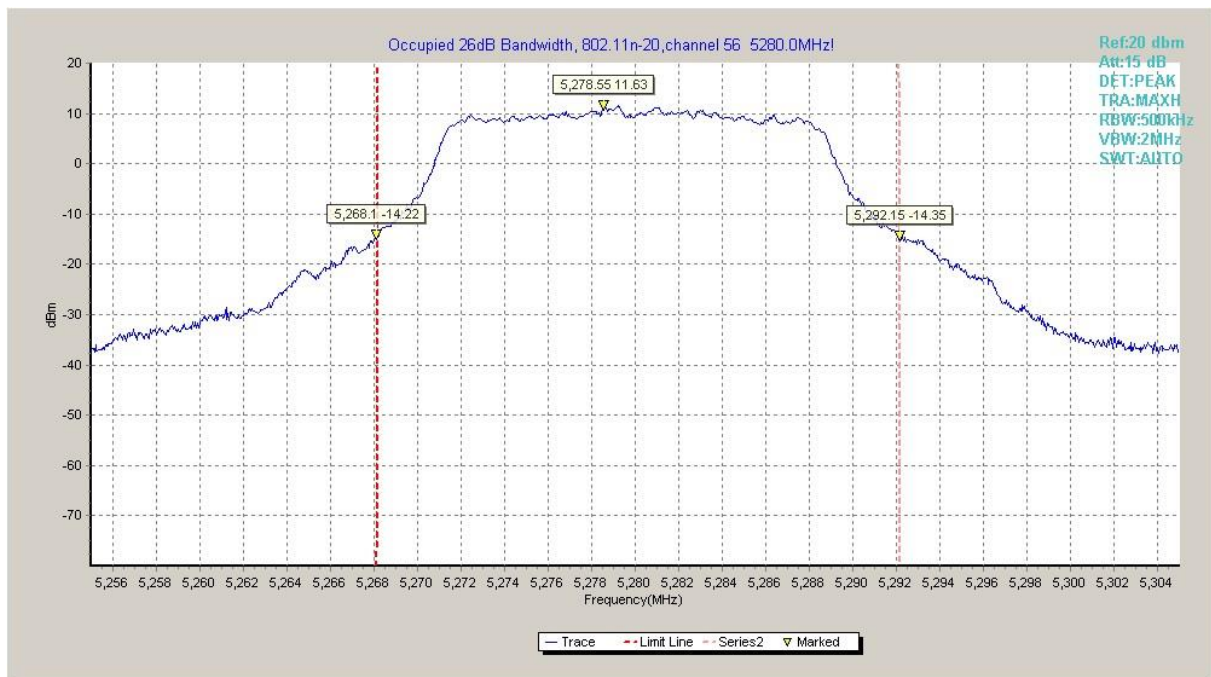
Fig.15 Occupied 26dB Bandwidth (802.11n-HT20, 5280MHz)
