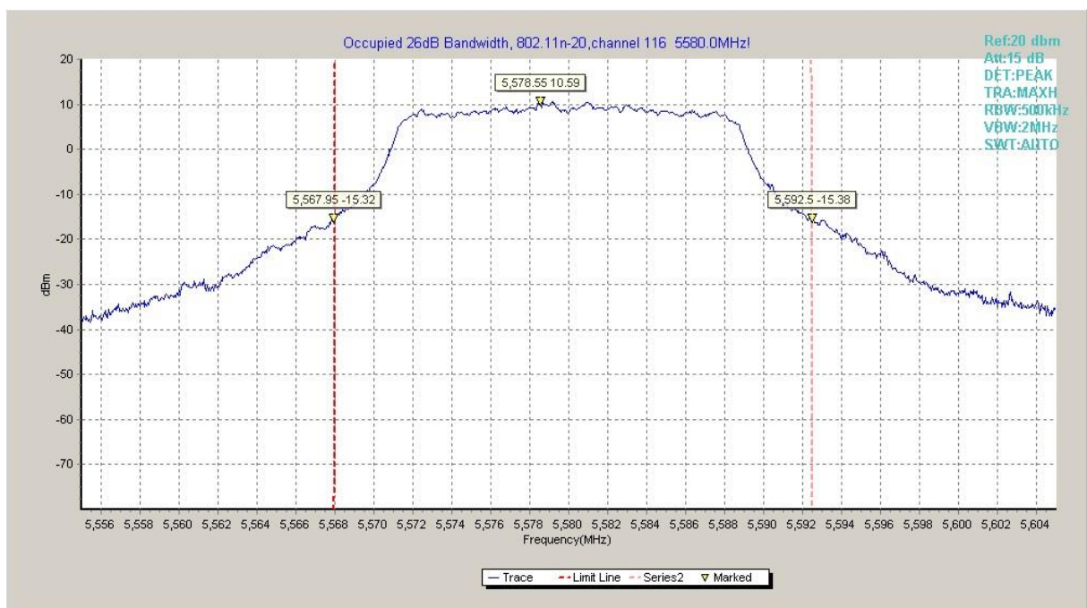
Fig.18 Occupied 26dB Bandwidth (802. 11n-HT20, 5580MHz)
