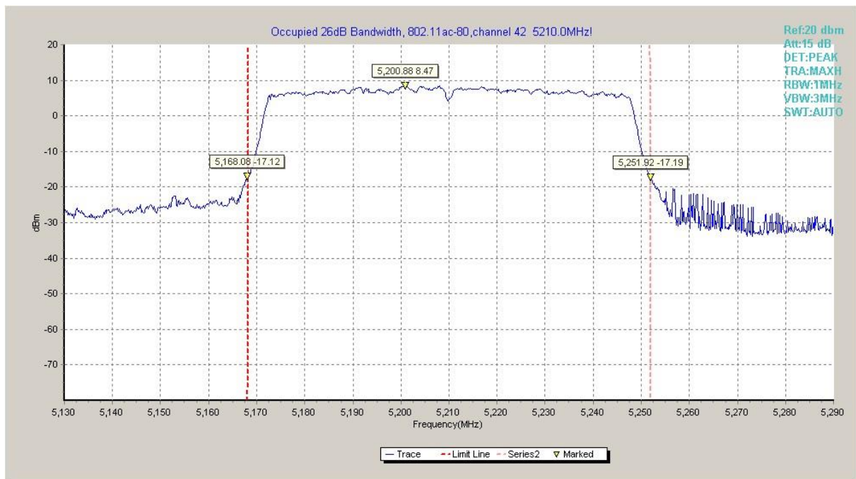
Fig.47 Occupied 26dB Bandwidth (802. 11ac-HT80, 5210MHz)
