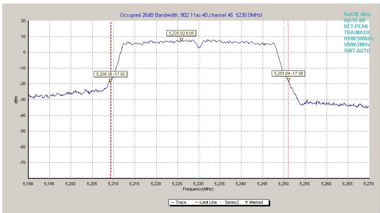
Fig.40 Occupied 26dB Bandwidth (802.11ac-HT40, 5230MHz)
