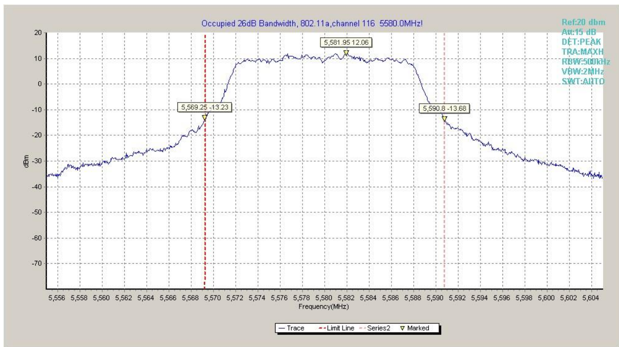
Fig.8 Occupied 26dB Bandwidth (802.11a, 5580MHz)
