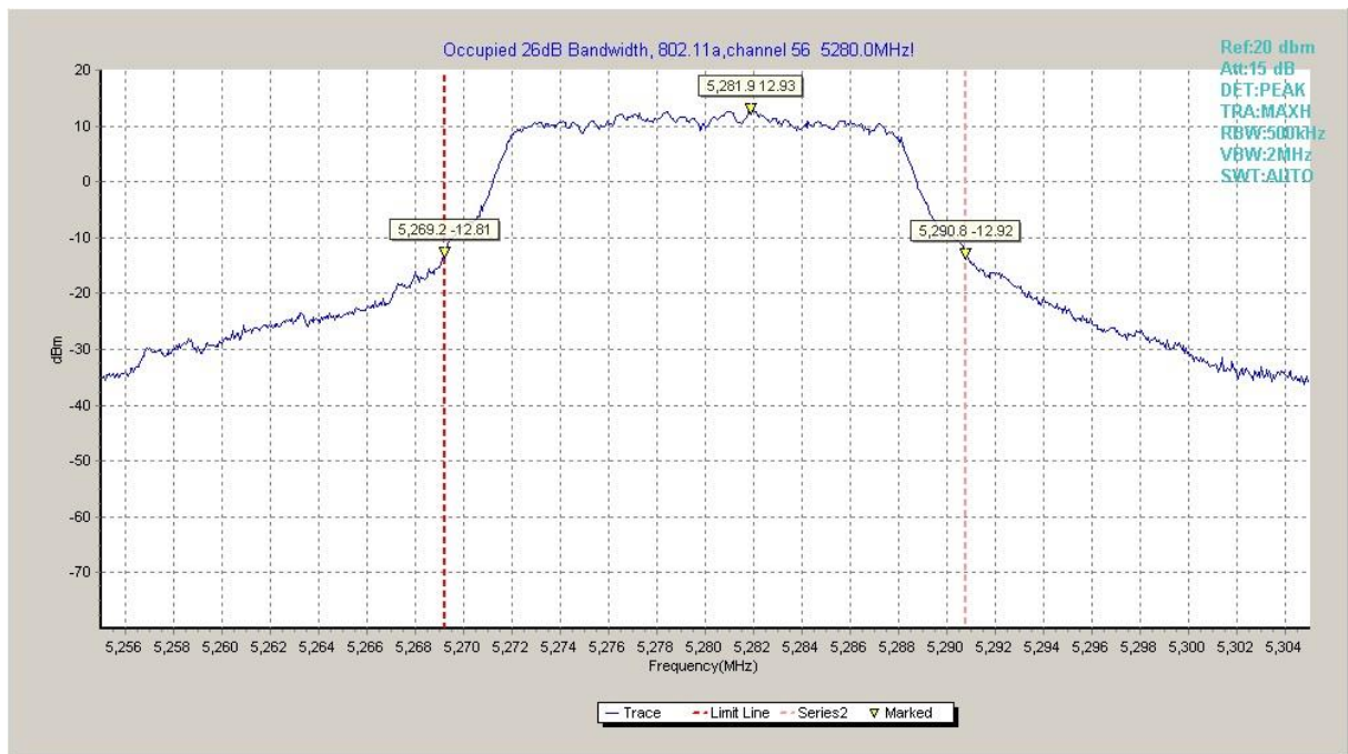
Fig.5 Occupied 26dB Bandwidth (802.11a, 5280MHz)
