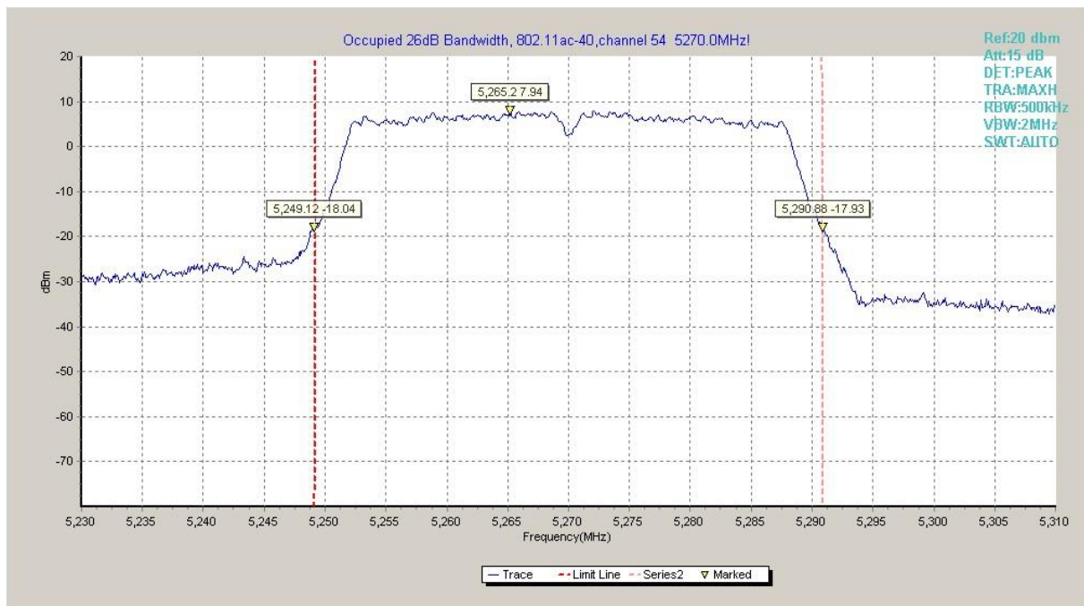
Fig.41 Occupied 26dB Bandwidth (802.11ac-HT40, 5270MHz)
