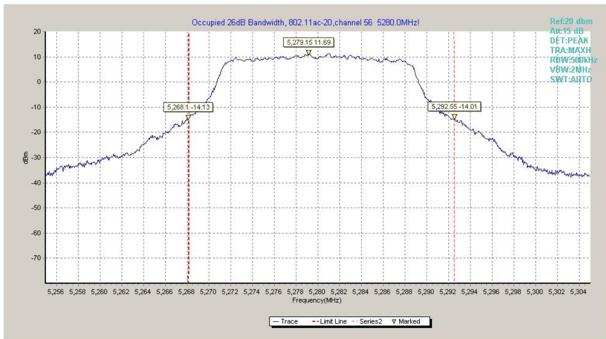
Fig.25 Occupied 26dB Bandwidth (802.11ac-HT20, 5280MHz)
