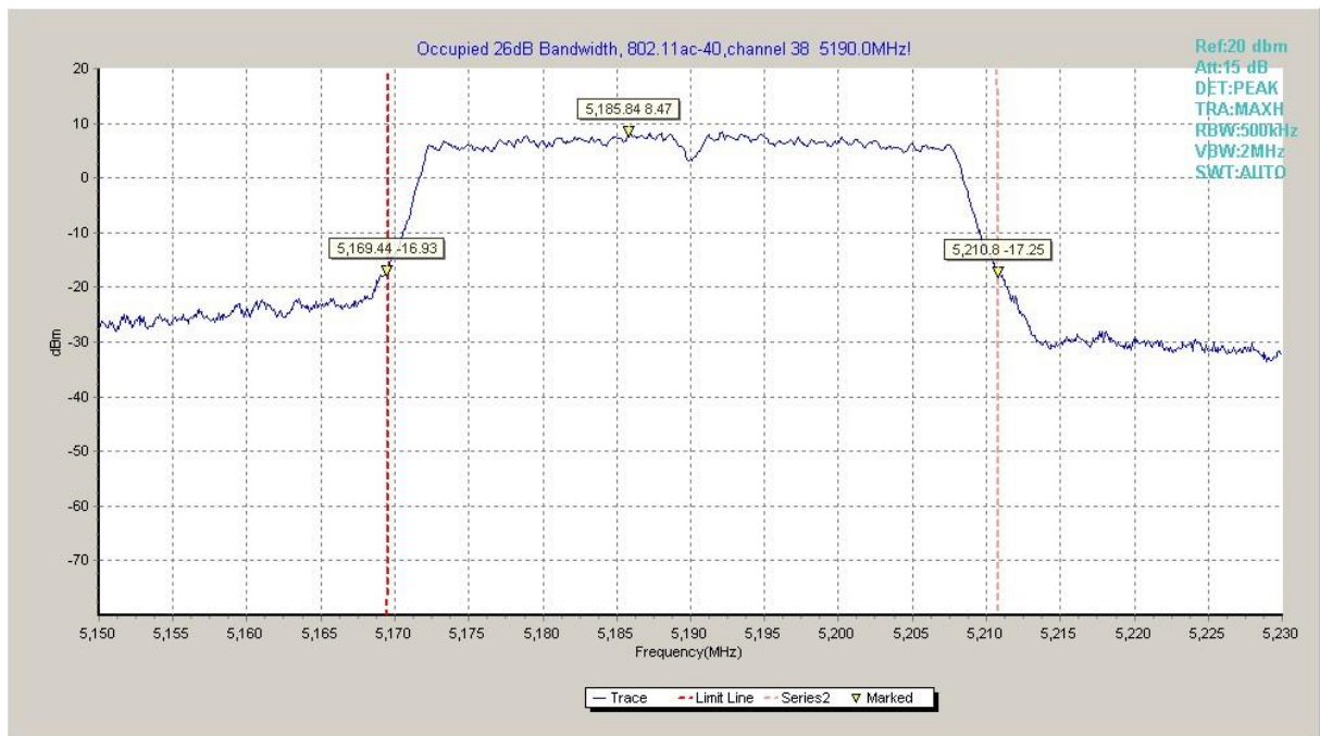
Fig.39 Occupied 26dB Bandwidth (802.11ac-HT40, 5190MHz)
