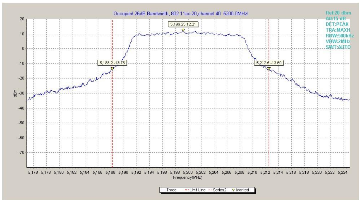
Fig.22 Occupied 26dB Bandwidth (802.11ac-HT20, 5200MHz)
