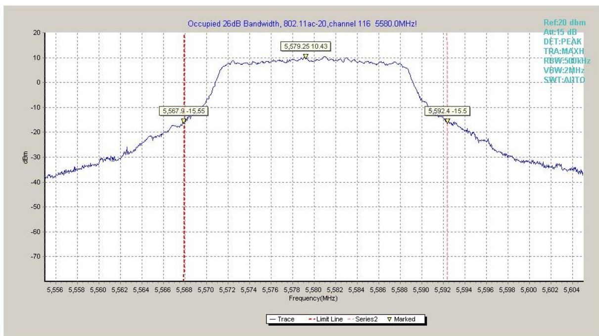
Fig.28 Occupied 26dB Bandwidth (802. 11ac-HT20, 5580MHz)
