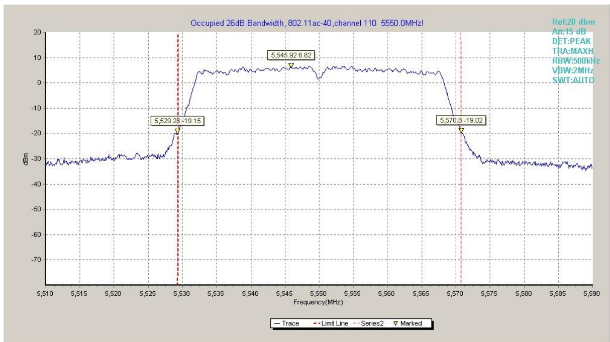
Fig.44 Occupied 26dB Bandwidth (802. 11ac-HT40, 5550MHz)
