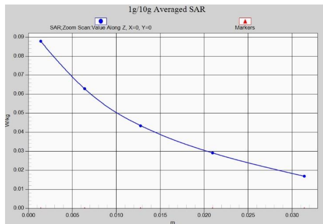
Fig.A.1- 15 Z-Scan at power reference point (LTE band4)
