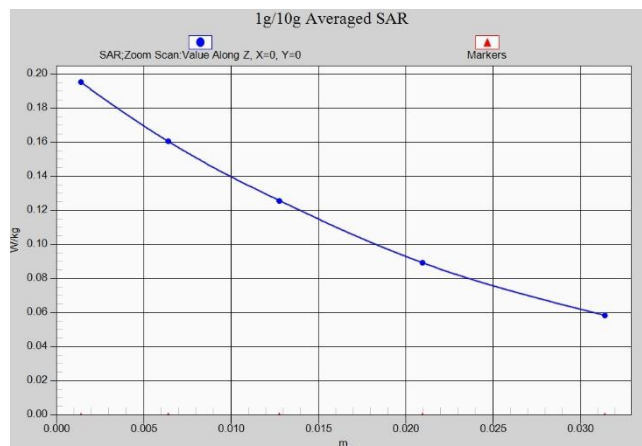
Fig.A.1- 21 Z-Scan at power reference point (LTE band26)
