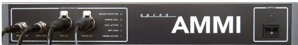
Figure 5.3 AMMI front panel
