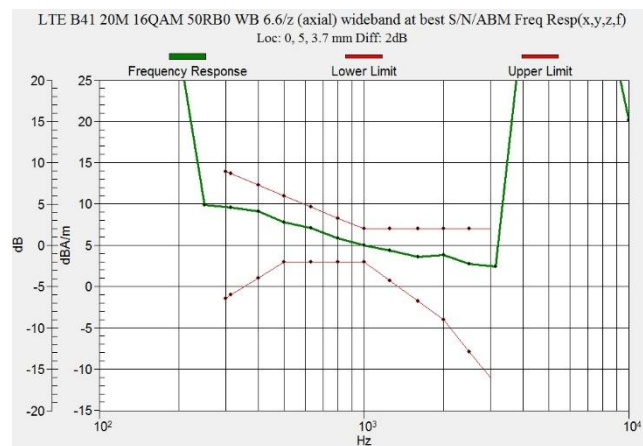
Figure C.12 Frequency Response of LTE B41 Power Class 2
