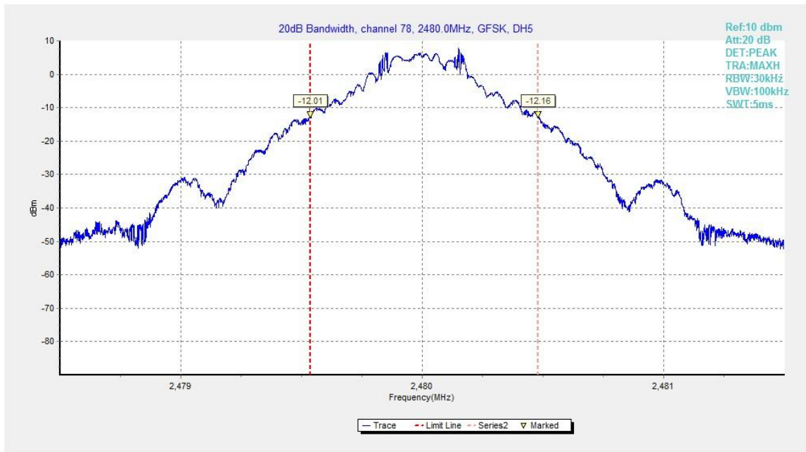
Fig.84. 20dB Bandwidth: GFSK, Channel 78
