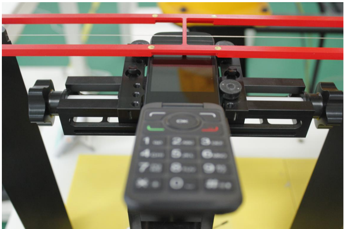
Picture 2: EUT Positioning for RF/T-coil
