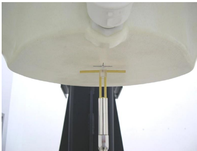
Picture 8.2 Photo of Dipole Setup
