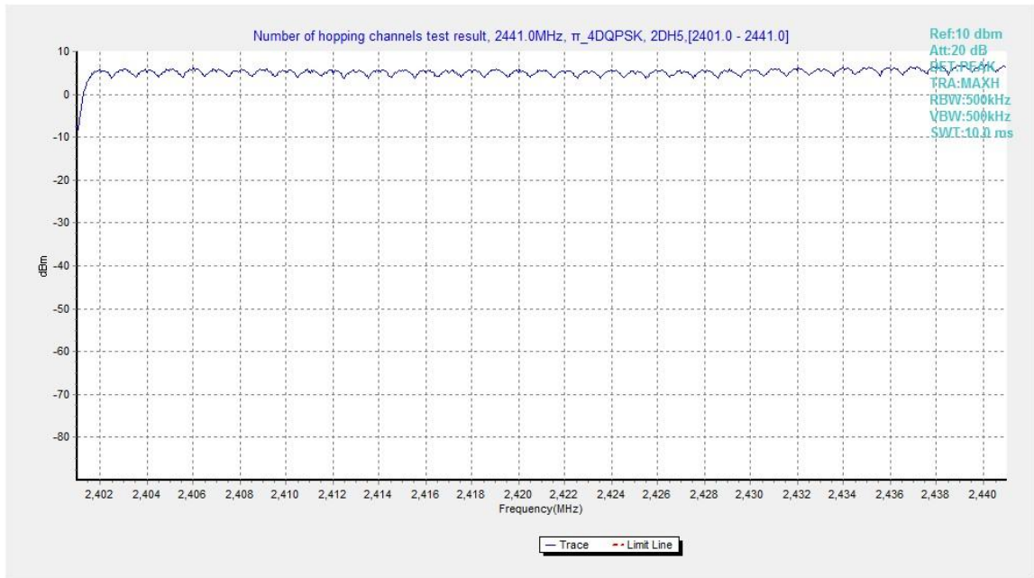
Fig.96. Number of hopping frequencies: \pi/4 DQPSK, Channel 0 - 39
