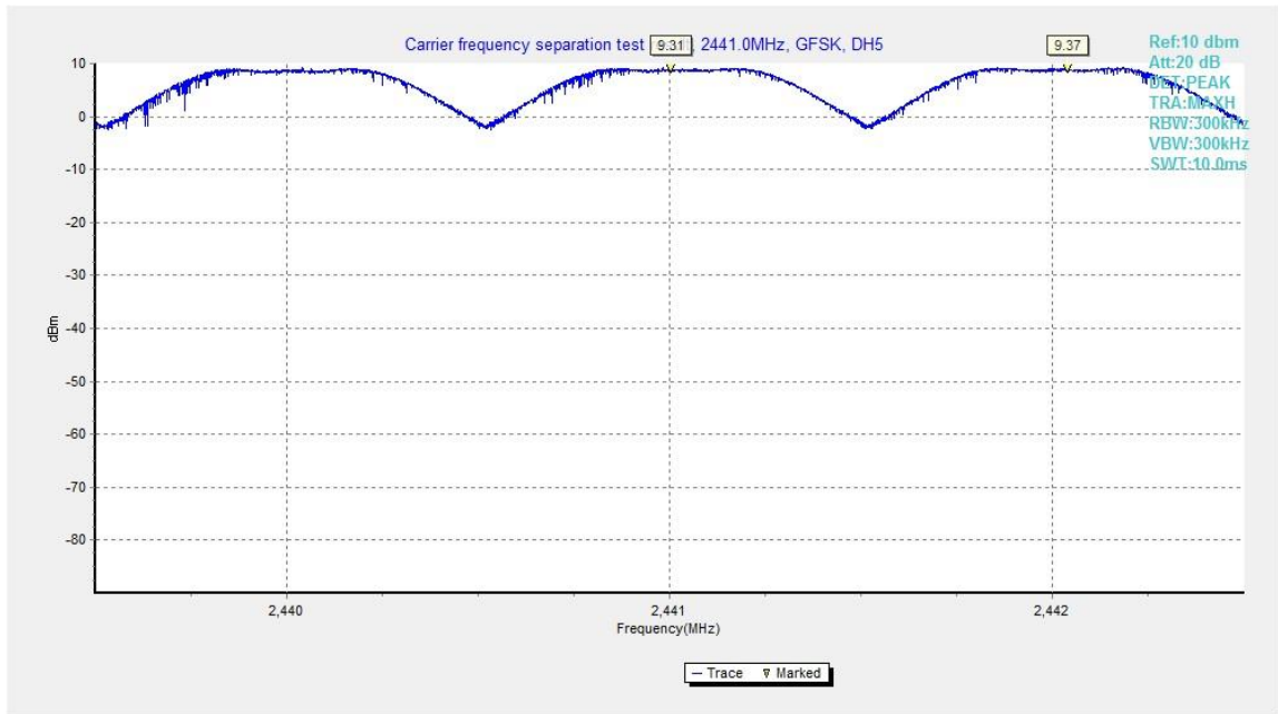
Fig.91. Carrier frequency separation measurement: GFSK, Channel 39
