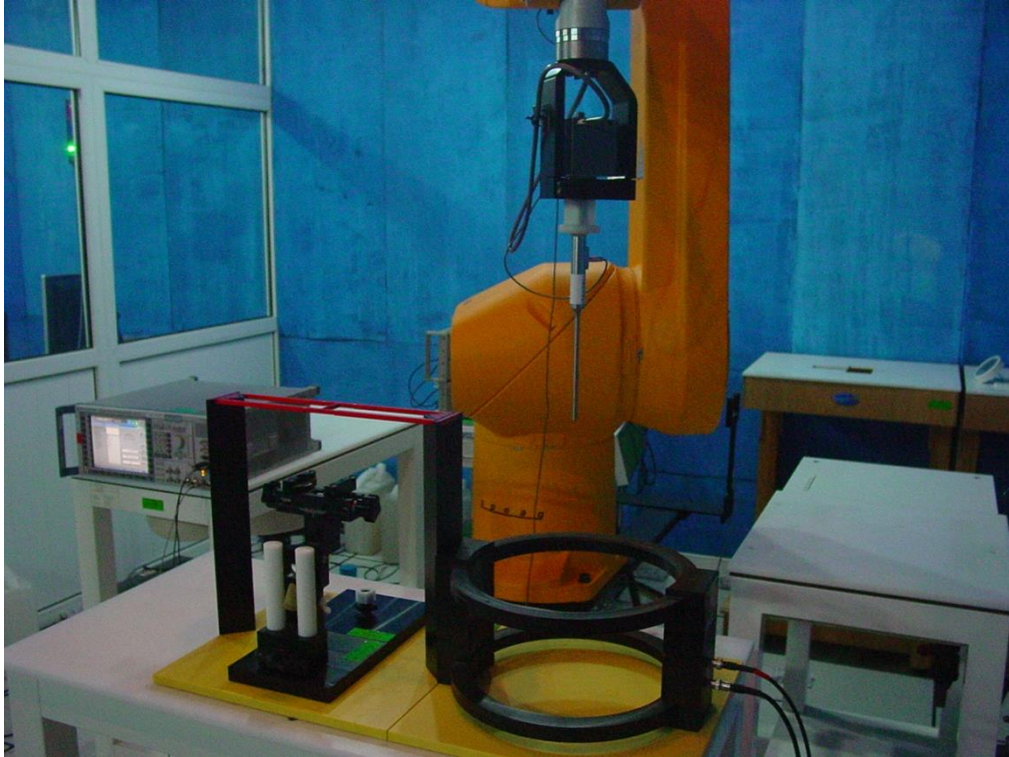
Picture A1: HAC T-Coil System Layout
