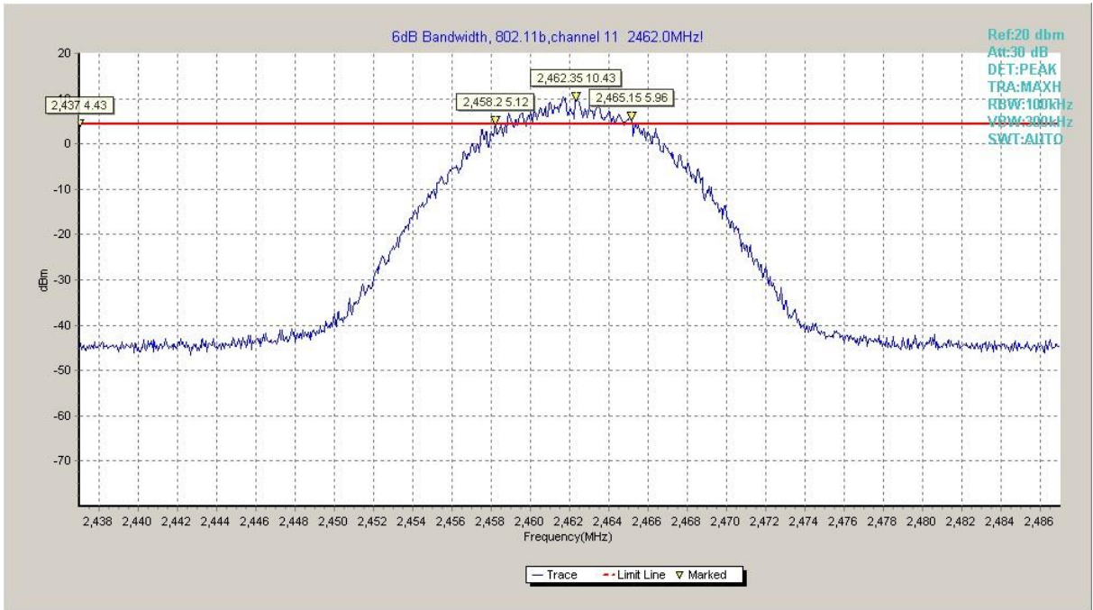
Fig.A.4.3 Occupied 6dB Bandwidth (802.11b, Ch 11)
