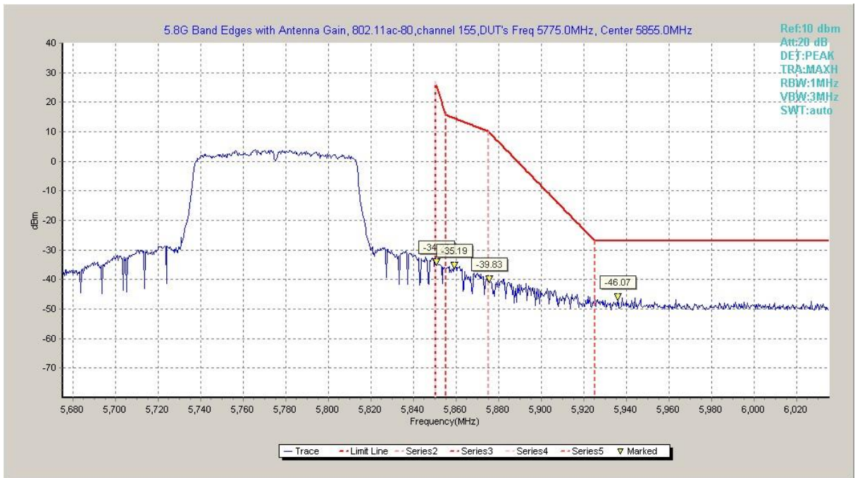
Fig. 82 Band Edges (802.11ac-HT80, 5775MHz)
