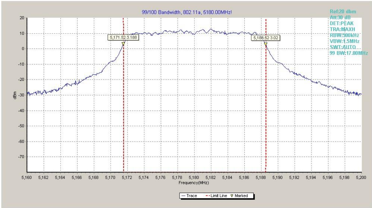
Fig. 71 99% Occupied bandwidth (802.11a, 5180MHz)
