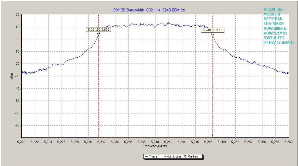
Fig. 73 99% Occupied bandwidth (802.11a, 5240MHz)
