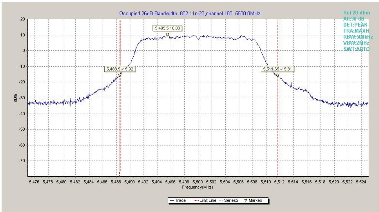
Fig. 16 Occupied 26dB Bandwidth (802. 11n-HT20, 5500MHz)
