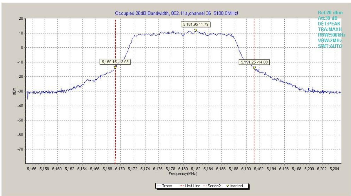
Fig. 1 Occupied 26dB Bandwidth (802.11a, 5180MHz)
