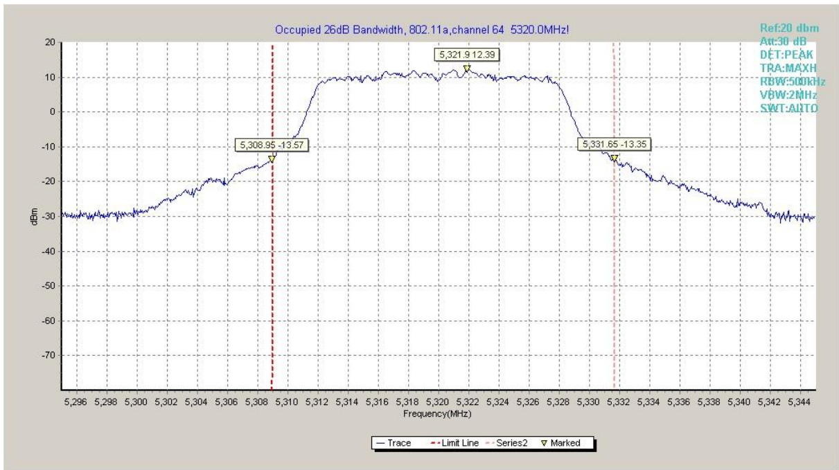
Fig. 6 Occupied 26dB Bandwidth (802.11a, 5320MHz)
