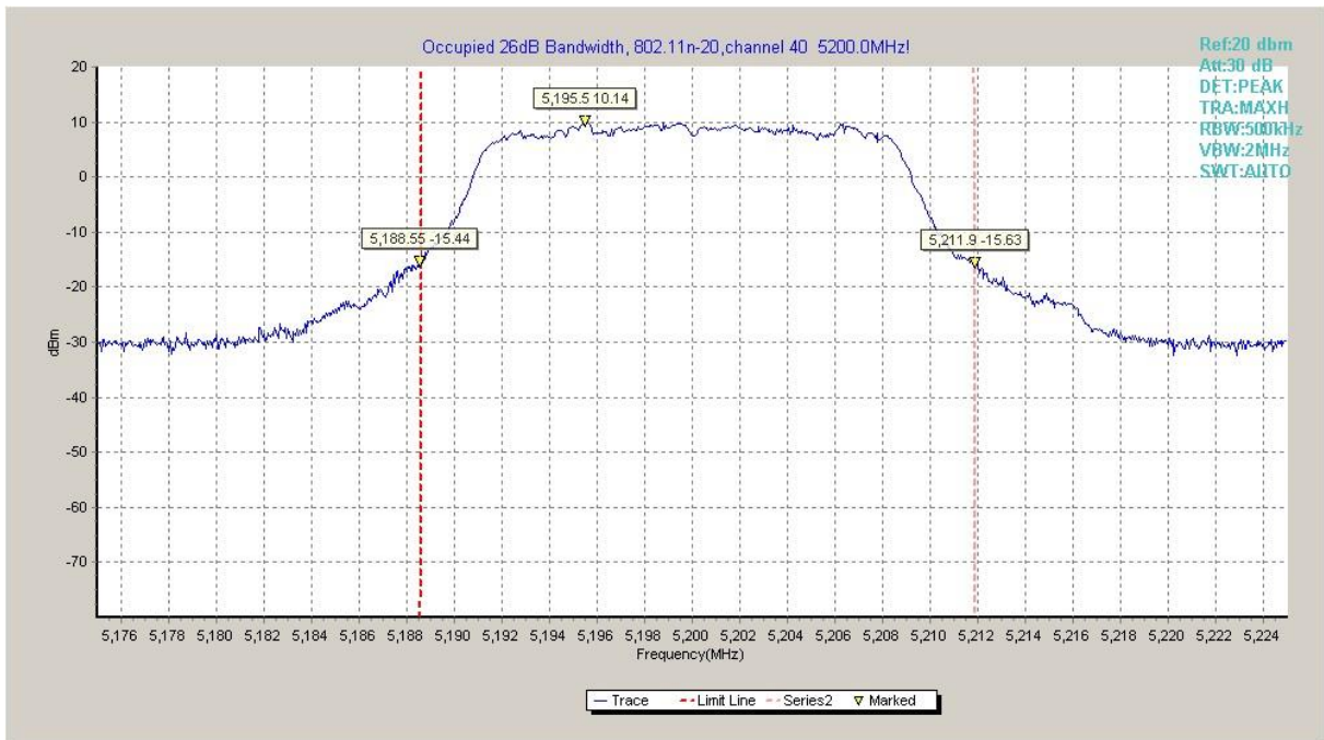
Fig. 11 Occupied 26dB Bandwidth (802.11n-HT20, 5200MHz)
