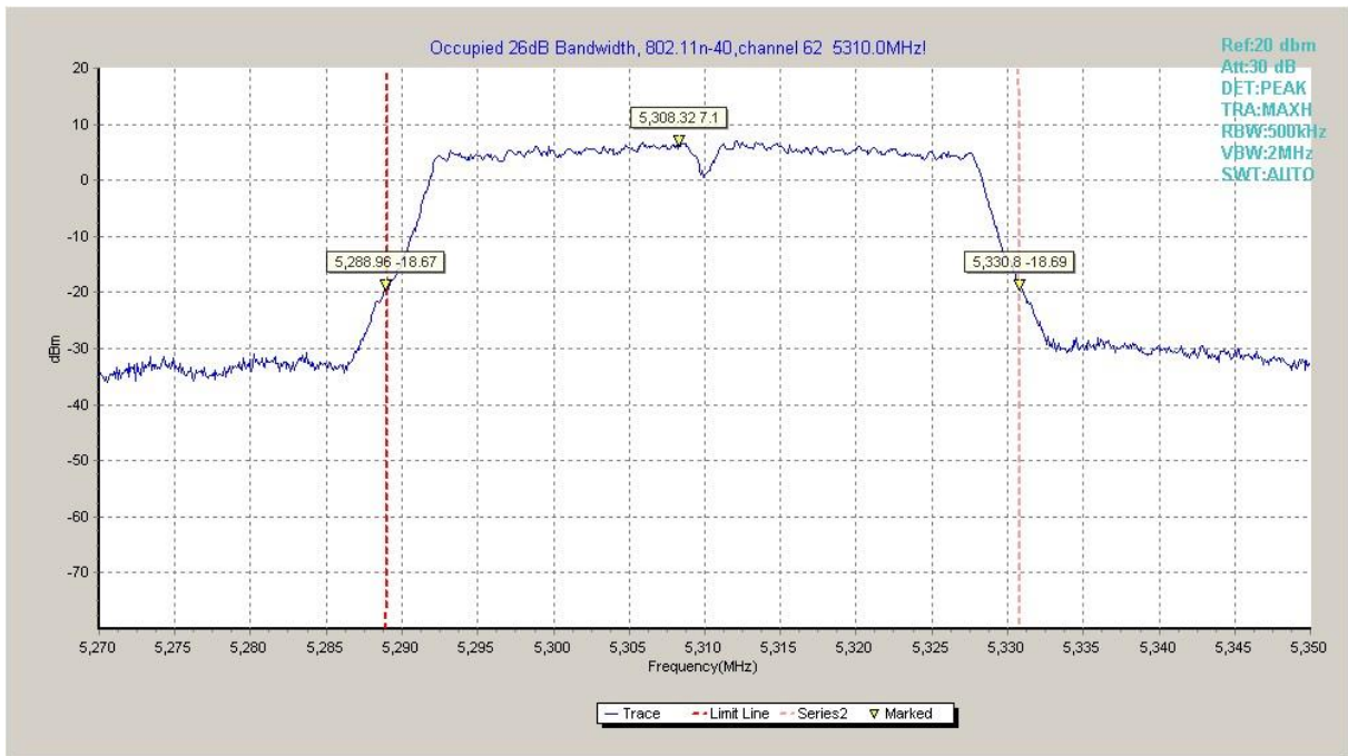
Fig. 31 Occupied 26dB Bandwidth (802.11n-HT40, 5310MHz)
