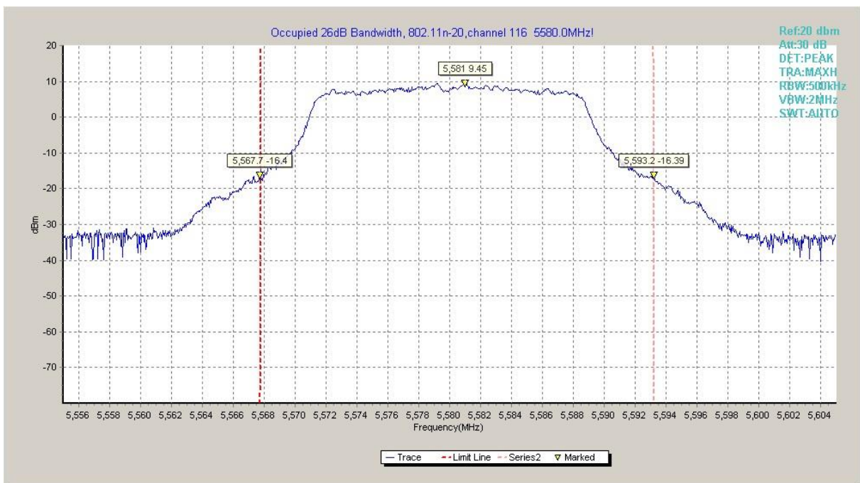
Fig. 17 Occupied 26dB Bandwidth (802. 11n-HT20, 5580MHz)
