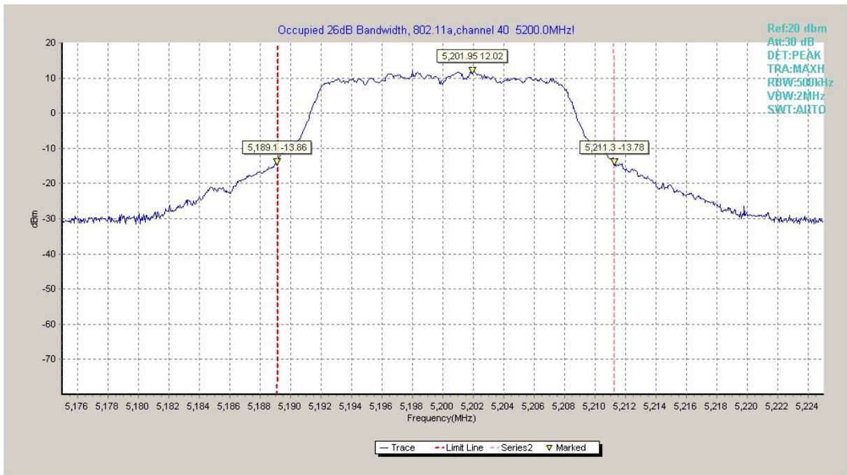
Fig. 2 Occupied 26dB Bandwidth (802.11a, 5200MHz)
