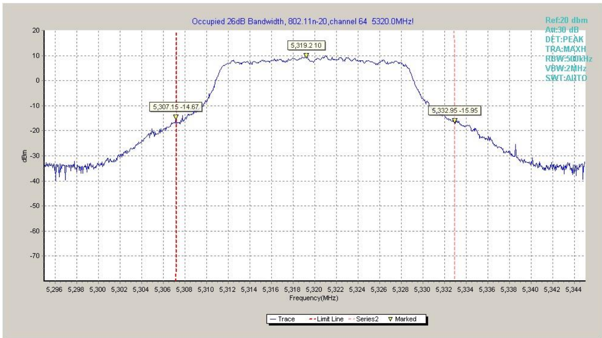
Fig. 15 Occupied 26dB Bandwidth (802.11n-HT20, 5320MHz)
